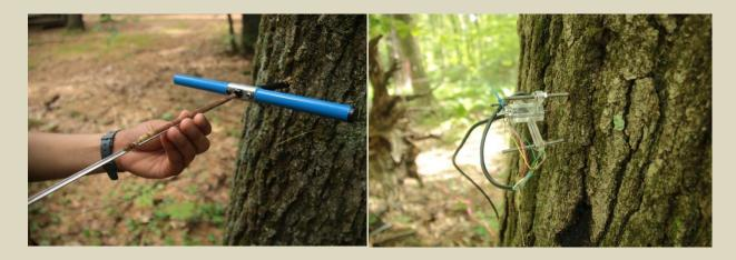
Dendrometers measure the tree's growth and provide insights into its health. Sensors measure sap and water flow within the tree's transport system to move water and nutrients. Photos by Shawna Greyeyes
